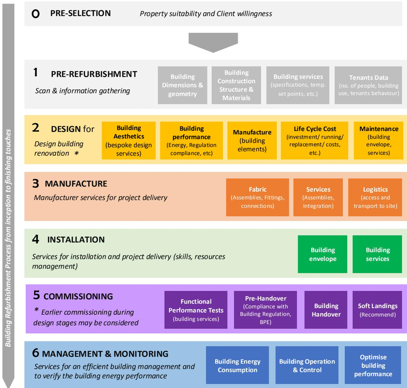
Figure 3-1 – Building refurbishment process.
