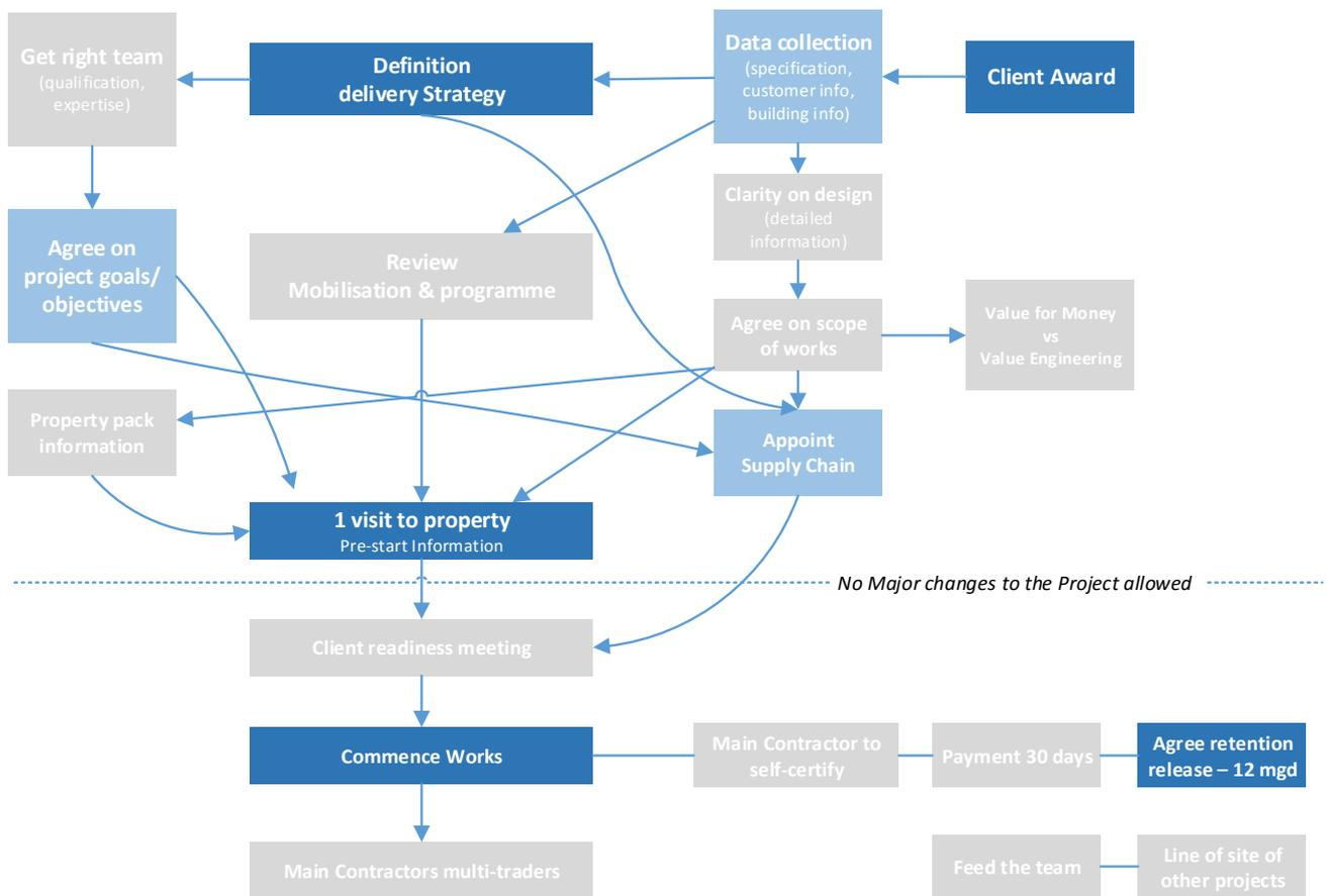
Figure 3-3 – Building refurbishment process – Main Contractor’s Perspective.
